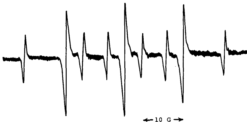
FIG. 9. ESR spectrum of the DMAO/PhG·H 2 O/BNO system after reacting at room temperature for 21 h in a 1:1 (v/v) MMA-acetonitrile mixture: [DMAO] = 1.5 \times 10^{-2} , [PhG·H 2 O] = 5.0 \times 10^{-2} , [BNO] = 5.0 \times 10^{-3} mol/L.
